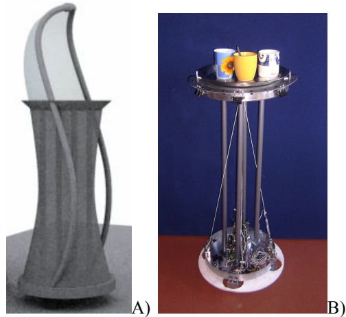
Figure 1. (A) CAD representation of ButlerBot. (B) Current state of the prototype. The tray has a height of 95cm.
