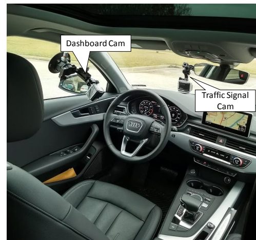
(c) Data collection setup inside the vehicle
